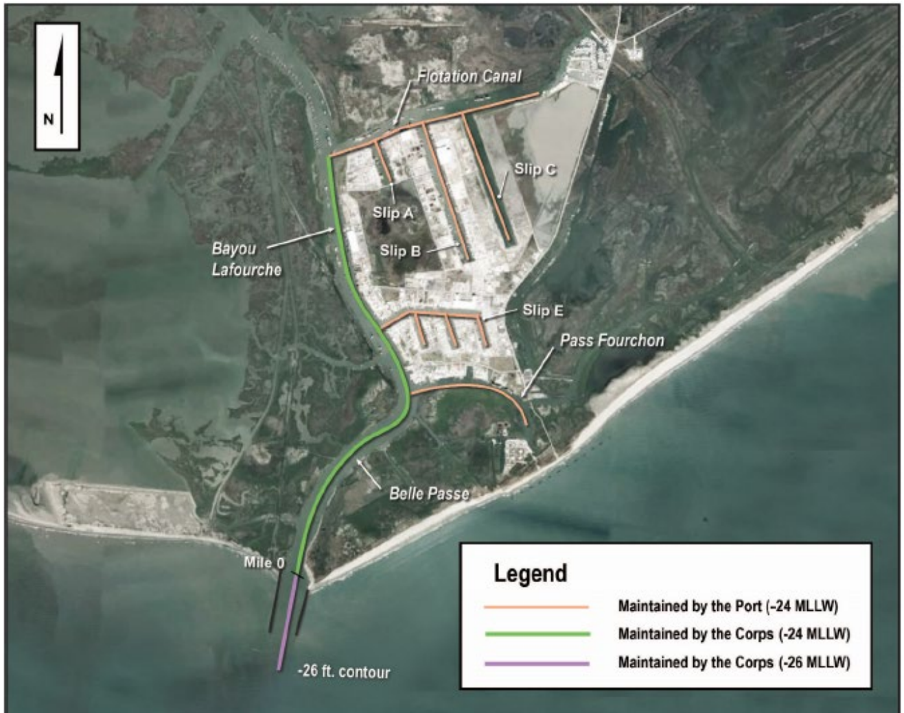
Figure 2. Map of the existing conditions at Port Fourchon, Louisiana at the mouth of Bayou Lafourche, Louisiana. The orange lines denote the slips and flotation canal maintained by the non-Federal sponsor: Greater Lafourche Port Commission. The green line denotes the inland reach maintained by USACE and the purple line denotes the offshore reach maintained by USACE.
