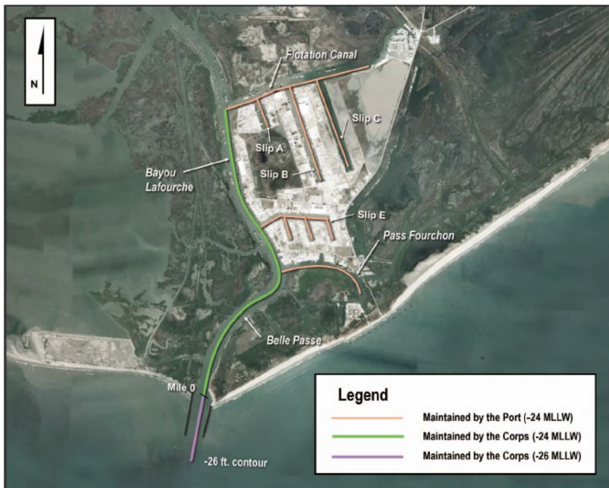
Figure 2: Project Area Map, green line is inland reach, purple line is offshore reach.
