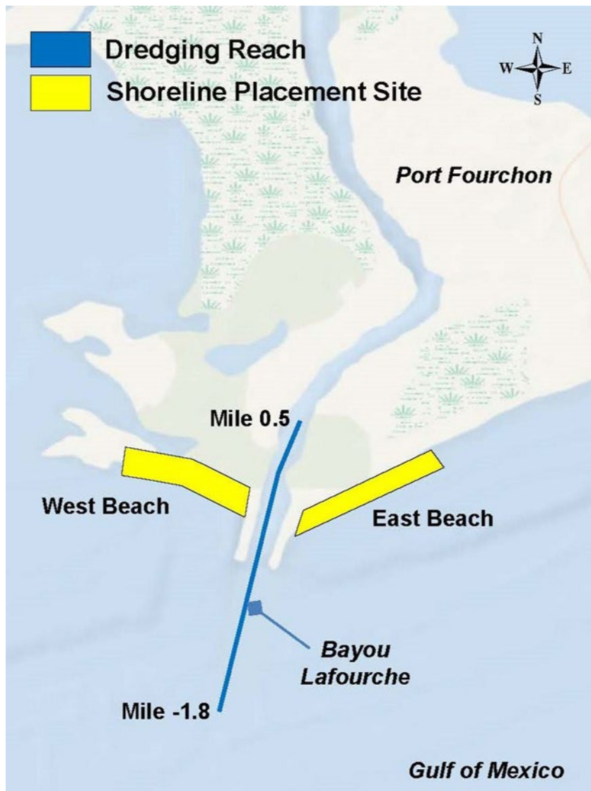
Figure 1. Proposed dredging and spoil placement for deepening of the Port Fourchon navigation channel.
